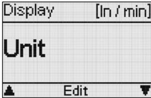
You can select the unit for the displayed measured value: l/sec, l/min, l/h, m³/h or gal/h.
