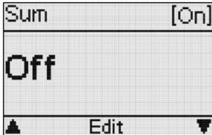
You can deactivate the summation function at any time. The display then shows the current flow rate in the required unit (see **Selecting unit**, page 14).
