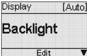
You can permanently switch on (**On** option) or switch off (**Off** option) the display backlighting. By selecting the **Auto** option, the backlighting will switch on the first time a button is pressed and automatically switch off again after 20 seconds.
