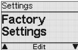
You can reset the device configuration to the factory settings, for example, in order to delete all data and settings simultaneously.
