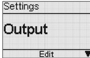
You can select the switching characteristic and the actuator for both switching outputs. After selecting the actuator, you have to define the threshold, at which the output changes its status.
