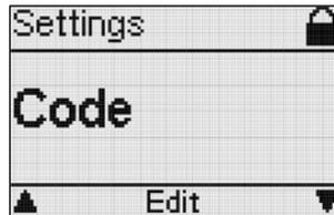
You can enter and activate a three-digit safety code to protect access to the device settings. The parameters and settings will then be visible but can only be changed after entering the correct code.
