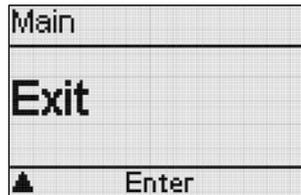
With the **Exit** function you can exit a menu or submenu and go to the next higher level.
