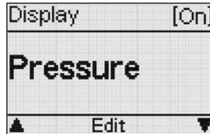
You can show (**On** option) or hide (**Off** option) the pressure in the display. The bottom left field in the display will remain blank if you switch off the pressure display,
